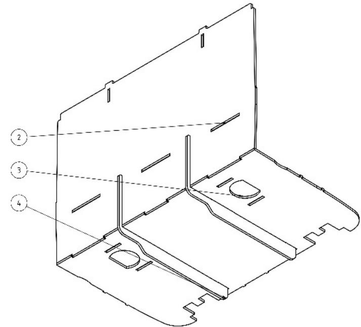
Glue the side parts (4) to the slots in part (3) right-angled and flush fitting and the dividing wall (2) also right-angled and flush fitting to the floor part (3).
