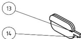
For orientation serves a stud at part (13) and (14), this must be exactly aligned at the front edge of the edge orientation. On the other hand, the part (13) is applied with (14) on the top of the "height jump".
