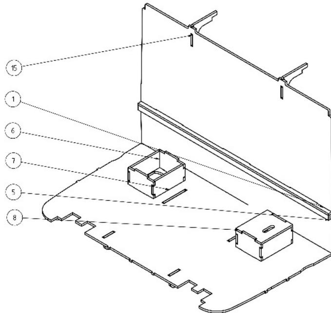
Put each dividing wall hook (15) in the respectively slit of the wall. See picture above.
