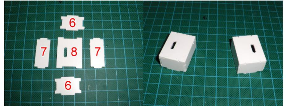
The two seat holder are placed on the module in the slots provided and glued in the correct orientation. The screw slots must lie outwards above the screw opening.
