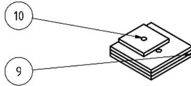
Assembly of the seat supporters (left and right). Use for that purpose the three plates (9) and a plate (10), layer them as shown and glue them to each other. Take as an alignment aid two pins. The holes initially serve only as positioning aid, later the hole under the small plates is used for screwing the seat to the seat base (see pictures below).
