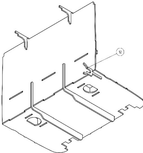
Glue the template (12) for the tilt limiter bearing with only some small glue points approx. 5 millimeters / 0.19 inch from the edge, after installation of the bearing it can later be removed again.
