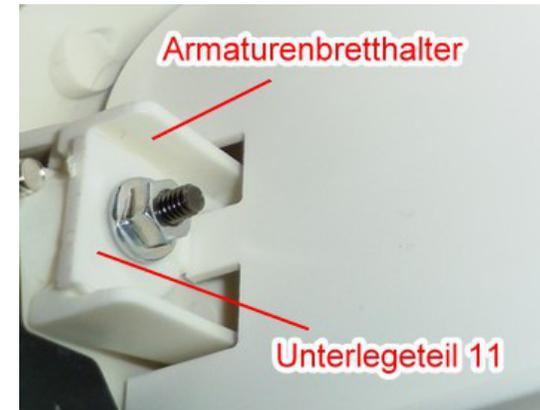
Since the original seat holders are not used, but are missing now as a rest for the collar nut of the dashboard holder, part (11) can be positioned below the collar nut one to the left and one to right. Thus, the dashboard holder is fixed now again.
