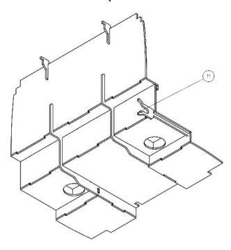
Glue the template (11) for the tilt limiter bearing with only some small glue points a approx. 5 millimeters / 0.19 inch from the edge, after installation of the bearing it can later be removed again.
