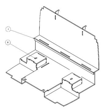
For visual enhancement of the two bars (7) can be glued now on the small rear wall (2) superimposed.
