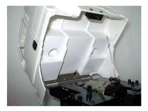
The cabin floor is now suspended from the bottom on the rear dividing hooks in the roof opening and launched forward along the body jaws (gently pressing enough). One sees above (fig. Similar) as the tilt limiter should be placed. Then the floor is screwed to the seat holders - done.
