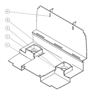
The two seat parts bumps (5) are each laterally correct fitting inserted and fixed in the slots of the side parts (6) and in the fitting grooves of the bottom plate (3). Then the four of seat parts along (9) and the seat parts (10) are fitted to a rectangular wall system. Here the seat plates (8) can be used as construction aid.
