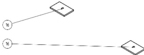
For a additional fixation of the drivers cab floor we have two plates (16) which be mounted below the original driver seat holder.
