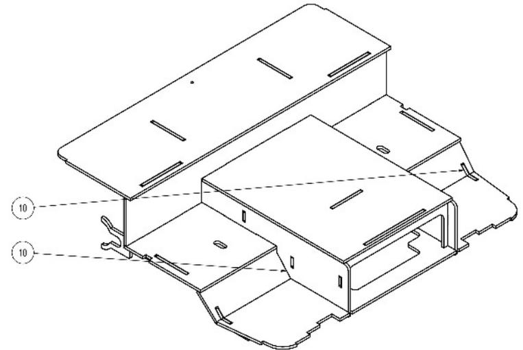
Mount the footwell parts (10) (left and right) between the side parts (2) and the joining aids (11) and (12) respectively.
