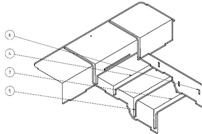
Fitting the support parts (4) to (6).
