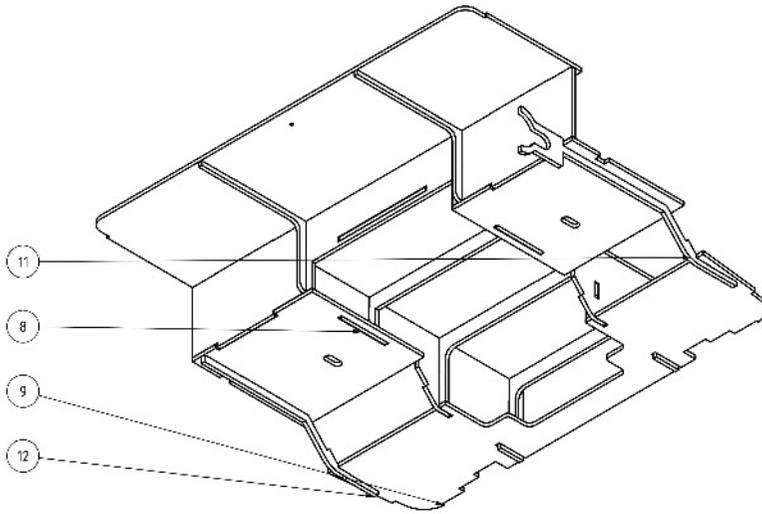
Mount the floor parts (8) (left and right) and the front cap floor (9) on the slots provided or respectively on the form elements, align and glue them together.
