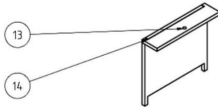
Assemble the rear support consisting of the two parts (13) and (14) and glue it to the center dome into the cab (possibly glue only one small point or secure it with double sided tape - see picture below).
