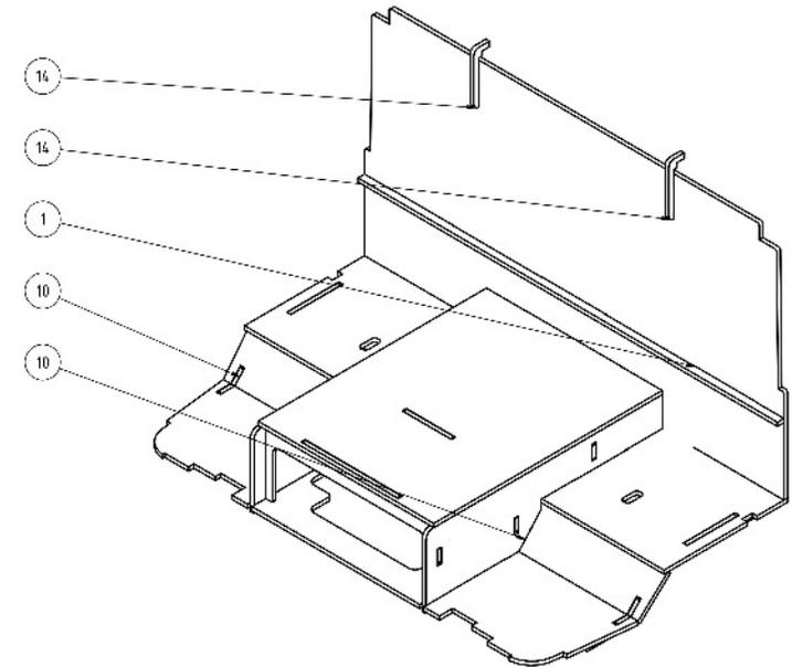
Mount the footwell parts (10) (left and right) between the side parts (2) and the joining aids (11) and (12) respectively.
