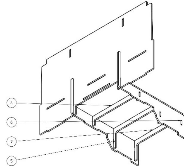
Fitting the support parts (4) to (6).
