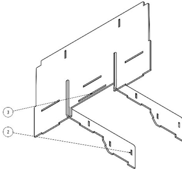
Glue the side parts (2) to the dividing wall (3) right-angled and flush fitting. The slots in part (3) would be helpful for this action
